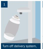
Turn off delivery system, remove and empty the water bottle.
