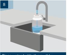
Rinse water bottle thoroughly. Refill bottle with water and flush through DUWL until empty.
