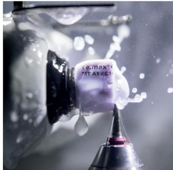
scanner and sets its approach. All of a sudden the cube starts spinning, the water starts squirting and the tool begins its slow precision cutting of the block.”
