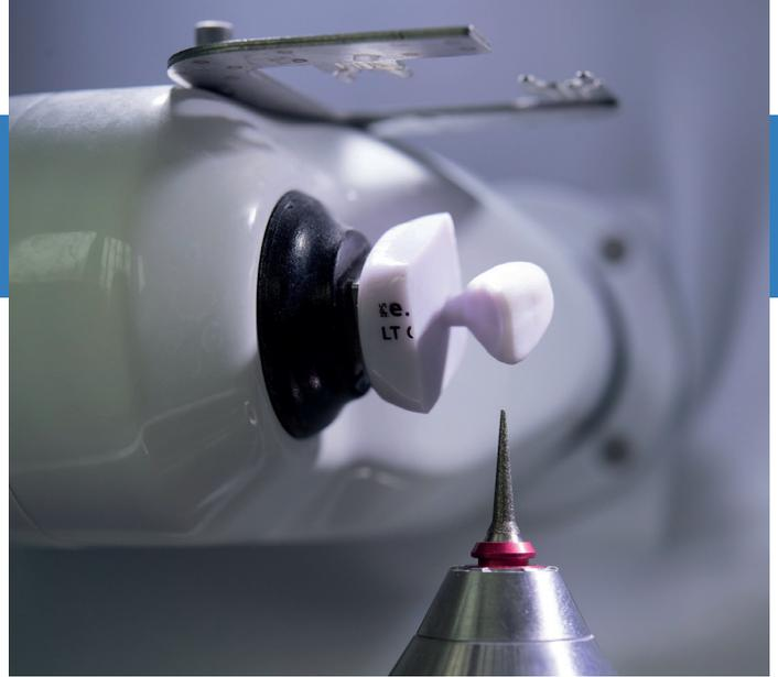
leave the block during the process, it decreases the crack propagations that often happen with other mills. Material and margin integrity are considered first in this process, and that leads to increased accuracy.
